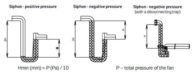
The air-handling unit can also be equipped with a siphon with a disconnecting trap and a ball valve (only negative pressure sections). This type of siphon need not be filled with water before putting it into operation. If there is a risk of freezing, it is necessary to insulate the siphon and condensate draining piping, respectively keep the ambient temperature above freezing point, e.g. with an electric heating cable!
