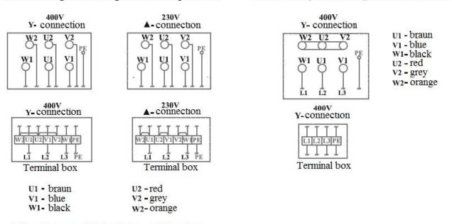
This schem provided only for 2.2 kW motors (max. power of 1~ frequency converter 2.2 kW)
