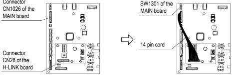
iv. Set the SW1301 of the MAIN board to ON condition before start the H-LINK operation (default position from factory is OFF condition).
